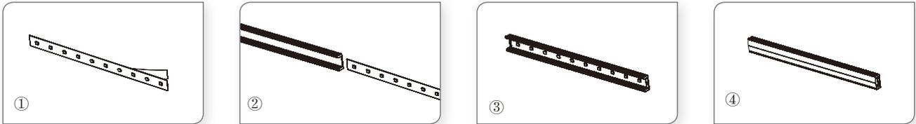
1. Peel away the self adhesive tape on the back of strip.
