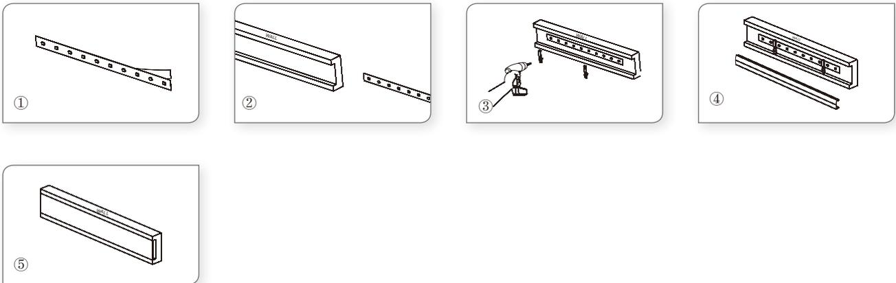
1. Peel away the self adhesive tape on the back of strip.
